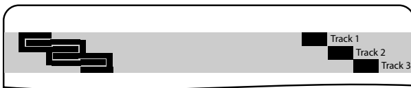
Figure 10: On the measurement card, a pattern of traces pass over read heads for detection. The black lines on the left indicate the pattern and position of the traces, which are aligned to the expected data track locations (shown on right for comparison). When a read head passes over the card, the traces are bridged and a circuit is completed. The traces are separated by 0.1 mm of space, which is over an order of magnitude smaller than the smallest read head we encountered.
