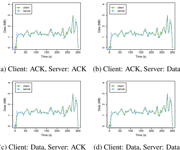
Figure 4: Asymmetric traffic analysis shows high correlation between a matched client/server pair
