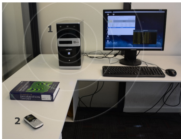
Figure 1: Demonstration of the covert channel in a working environment. Signals at GSM frequencies are emitted from the workstation and received by the nearby compromised mobile phone.
