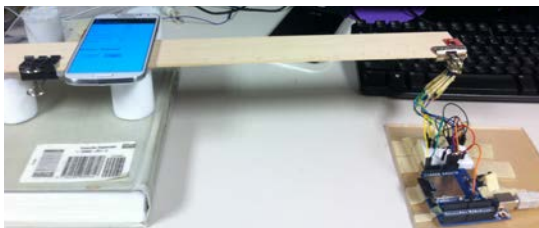
Figure 9: Cantilever based receiver platform for vibration amplification.
