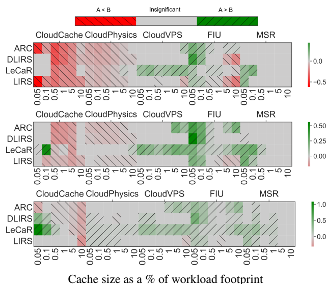
Figure 8: Paired t-test analysis to understand the difference in performance between (A) CACHEUS vs. (B) Other. The three panels compare four “Other” algorithms (i.e., ARC, DLIRS, LeCaR, and LIRS) against the following variants of CACHEUS: Top: C1, Middle: C2 Bottom: C3. Green colors indicate that the CACHEUS variant was significantly better, red colors indicate that the CACHEUS variant was significantly worse, and the gray color indicates no significant difference. Brighter green and red colors indicate higher effect sizes. Effect sizes were computed using Cohen’s d -measure.
