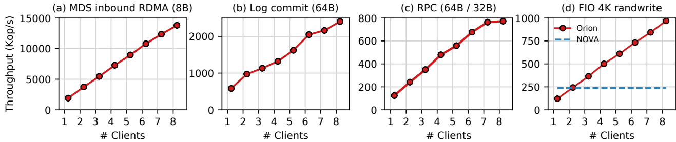
Figure 10: Orion metadata scalability for MDS metadata operations and FIO 4K randwrite Orion exhibits good scalability with rising node counts for inbound 8 B RDMA reads (a), 64 B log commits (b), RPCs (c), and random writes (d).
