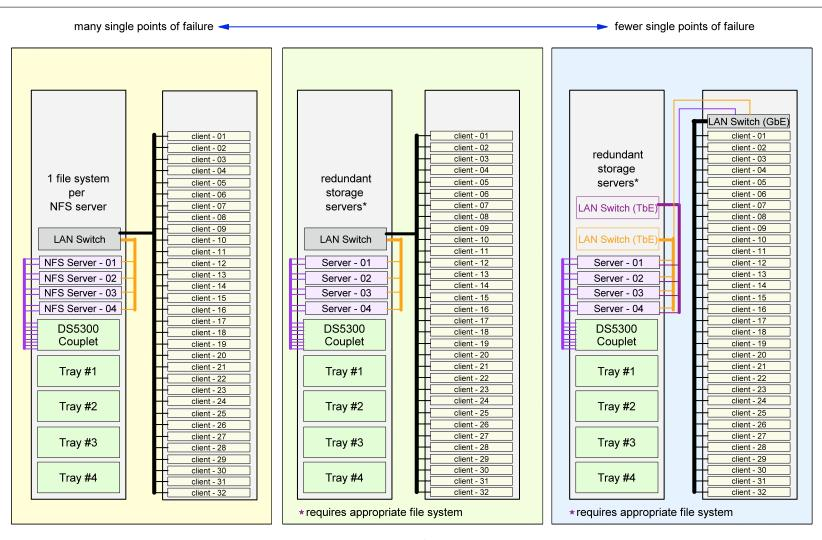
Increased redundancy can be achieved using 2xGbE per client and distributing the cluster over multiple sites. Carefully assess uptime requirements to avoid "gold plating" in this regard.
