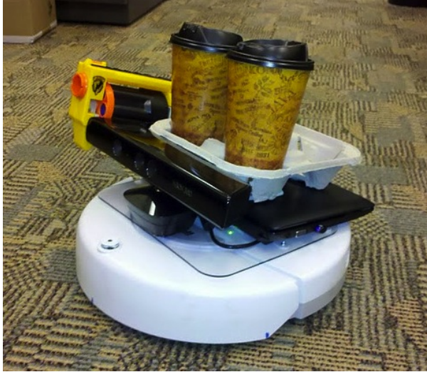
Figure 1: Our experimental robot platform. To experiment with secure robots we built a robot using an iRobot Create, a netbook running Linux, and a Kinect for extra sensing.
