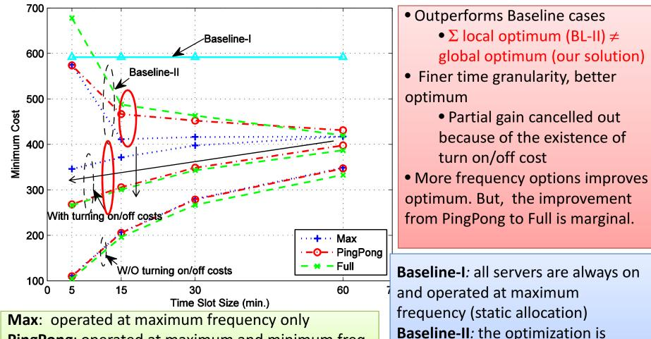
**PingPong**: operated at maximum and minimum freq. **Full**: operated at full spectrum (discrete)
